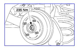
2. **CAUTION:** Rotate the brake drum 10 times in the opposite direction when tightening the wheel hub retaining nut to prevent damage to the bearing.
