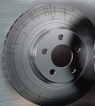
High Amounts of Cracking In Extreme Driving Conditions.
