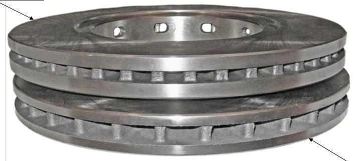
\*Plate Thickness DOES NOT Meet OE Manufacturer Specification \*25% Fewer Cooling Vanes Competitor Rotor\*
